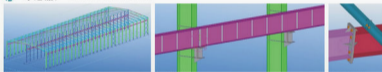
整体透视图 OVERALL PERSPECTIVE VIEW 吊车承载梁 SUPPORTING BEAM OF CRANE RAIL 梁梁连接 CONNECTION BETWEEN BEAMS
